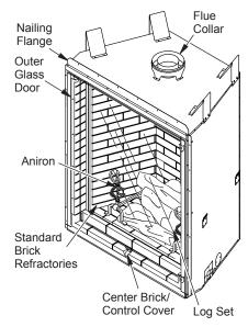
Figure 1 - Direct Vent Fireplace (DVF-36SC Shown)
